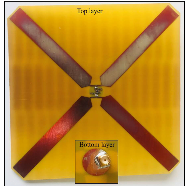
FIGURE 7. Developed planar printed cross dipole antenna for glacier surface receiver applications.
