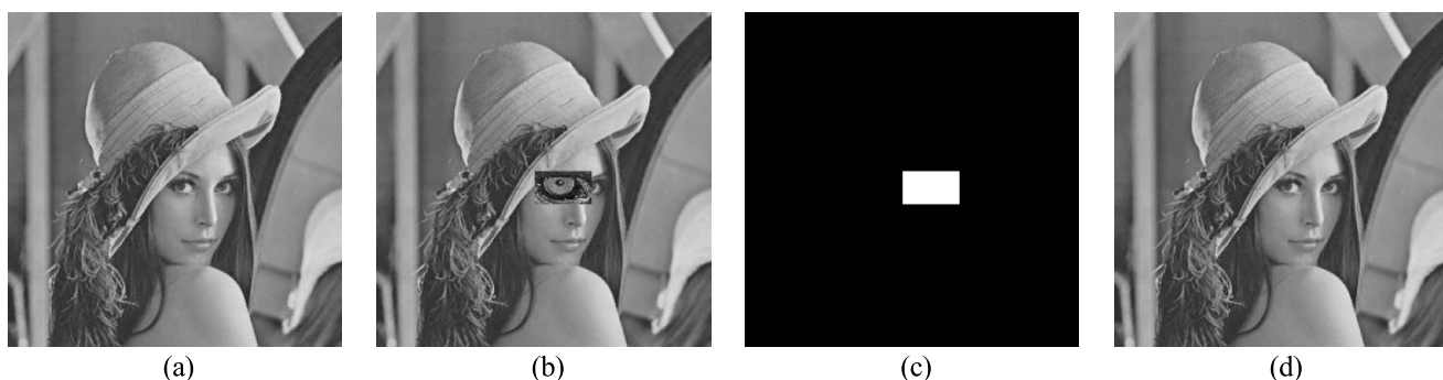
FIGURE 7. Sample of collage attack \approx 1.69\% ((a) watermarked image, (b) tampered image, (c) tampered area, (d) restored image).
