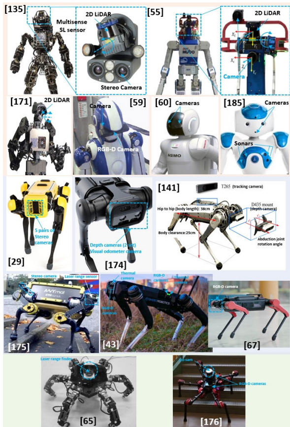
FIGURE 14. Examples of sensing systems used in legged robots for stair-climbing/detection.
