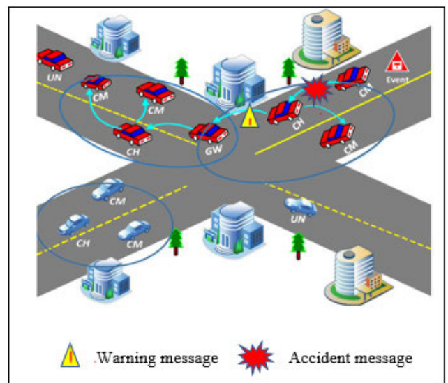
FIGURE 2. Emergency message communication.
