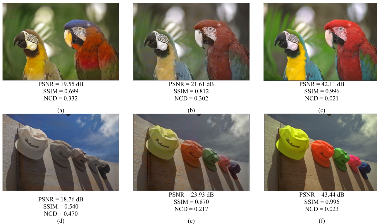
FIGURE 31. Colorized images obtained by (a), (b) deep colorization [40], [45] with no reference; (c), (d) deep colorization [40] with reference; and (e), (f) our proposal.
