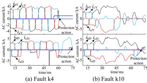
**FIGURE 2. Valve-side three-phase AC current waveforms for different faults.**
