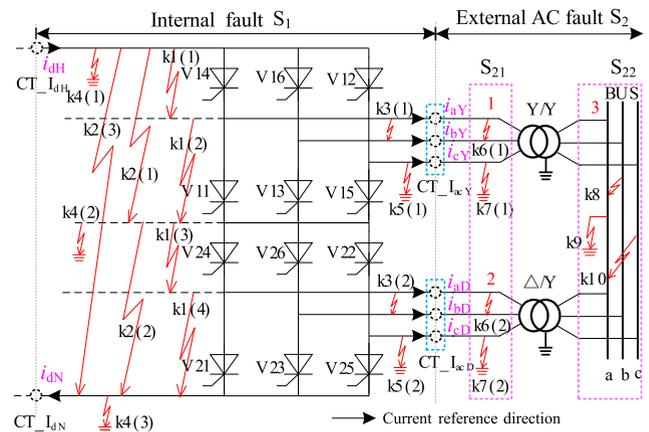
FIGURE 1. Converter fault distribution.
