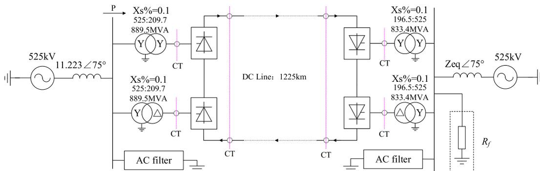
FIGURE 6. LCC-HVDC system model.
