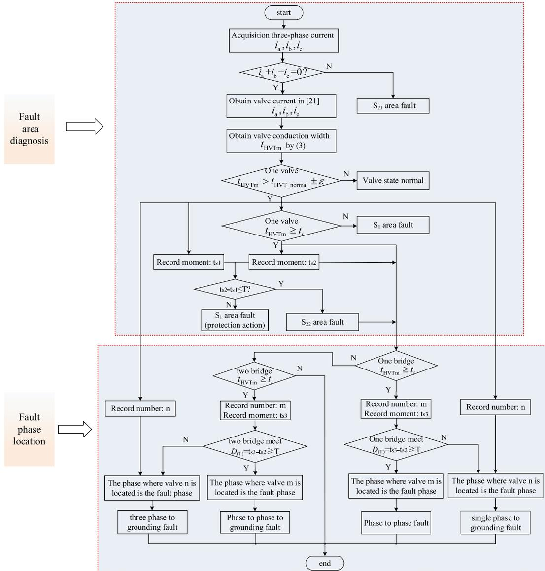
FIGURE 5. The flow chart of fault phase location.
