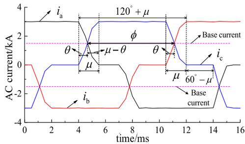
FIGURE 3. The AC current waveform during normal operation.
