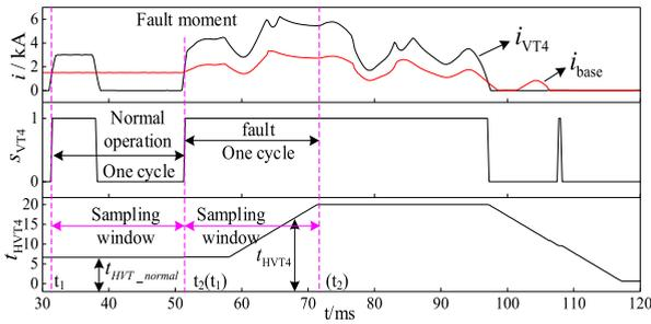
FIGURE 4. Converter valve current and conduction width waveforms.
