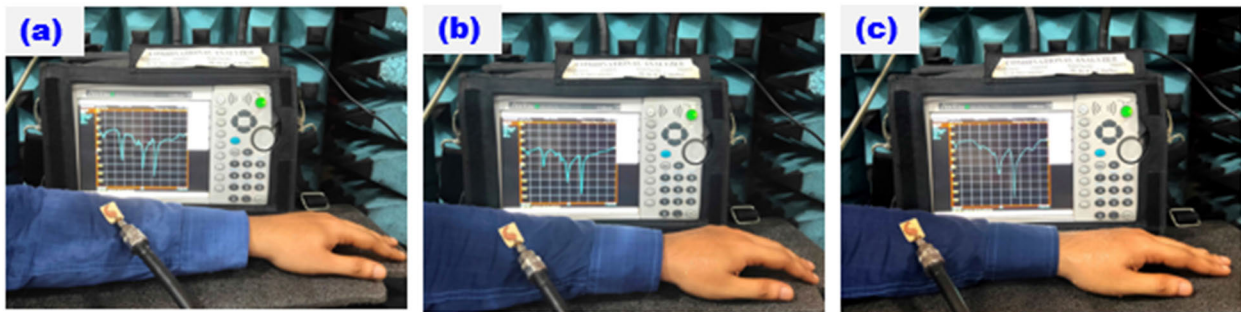
FIGURE 10. Measurement setup of the jute textenna in different on body human sweat environments (a) little exposure, (b) partial exposure, (c) complete absorptency.
