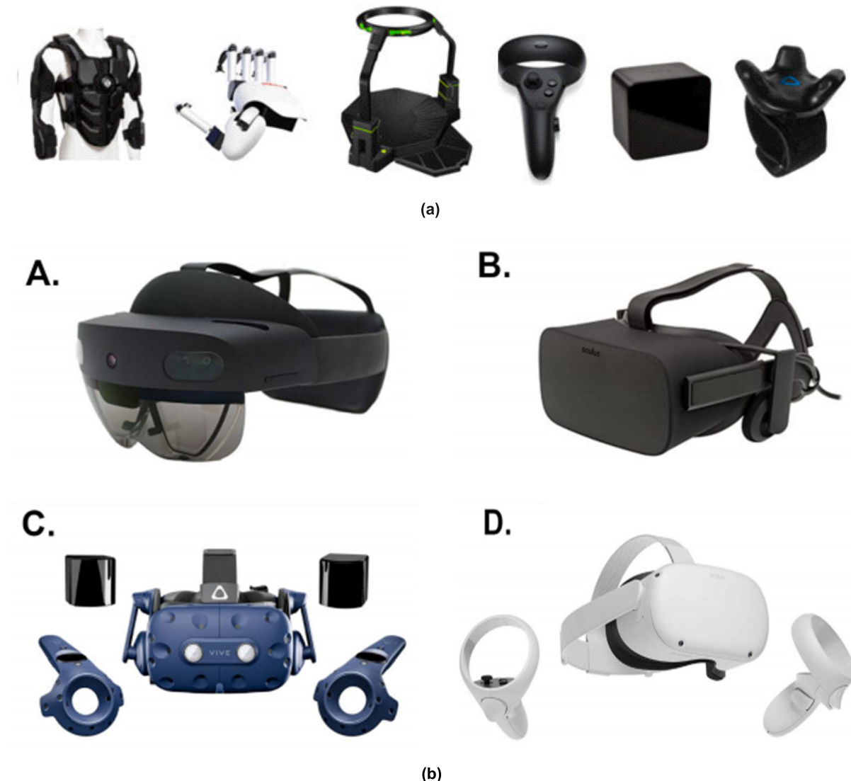
FIGURE 5. (a) VR accessories that provide an immersive experience (suit, haptic glove, omni-directional treadmill, motion sensor controller, lighthouse, tracker). (b) Popular VR Headsets: A. Microsoft HoloLens 2. B. Oculus Rift CV1. C. HTC Vive. D. Oculus Quest 2.
