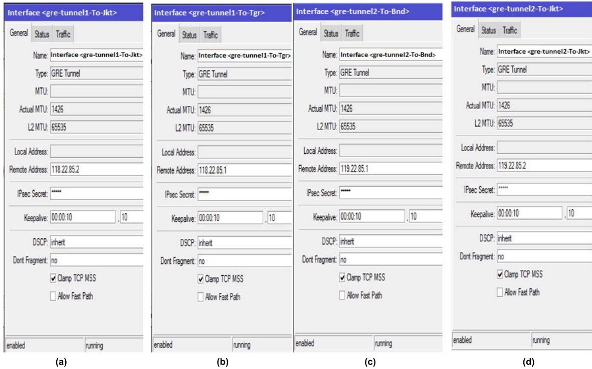
FIGURE 3. GRE+IPSec tunnel configuration.
