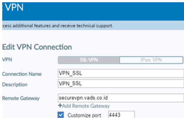
FIGURE 6. SSL VPN configuration.
