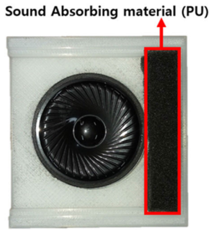
FIGURE 18. Experimental sample for test verification of sound-absorbing material application.
