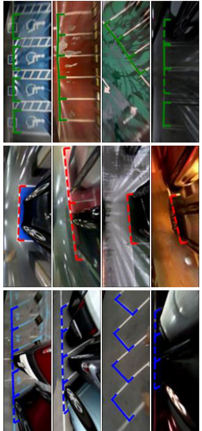
FIGURE 7. Parking slot detection results of the proposed method in various parking scenarios in the test images of the SNU dataset. The first, second, and third rows shows the detection results for perpendicular, parallel, and slanted parking slots, respectively. Green, red, and blue lines indicate perpendicular, parallel, and slanted parking slots, respectively; solid and dashed lines indicate vacant and occupied parking slots, respectively.
