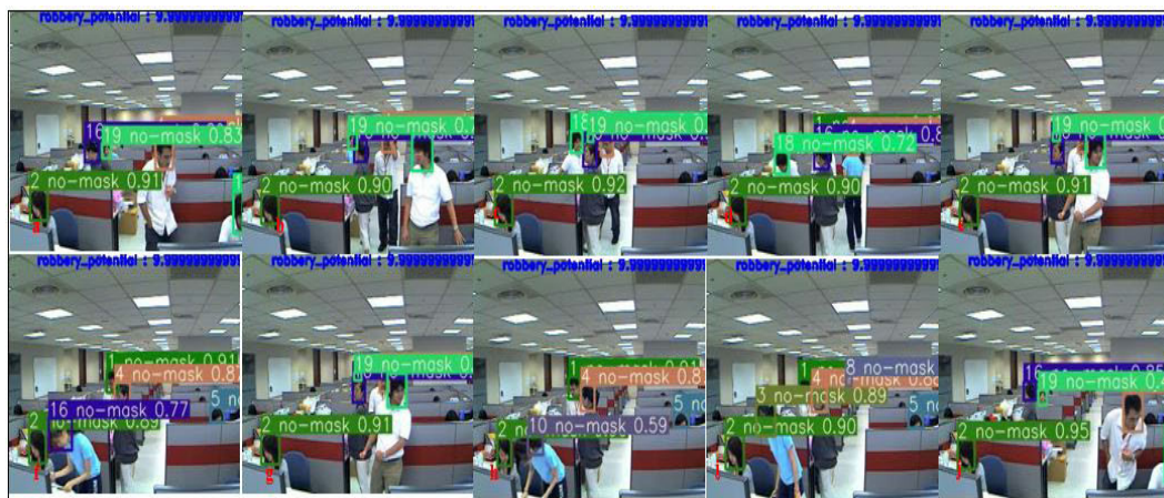
FIGURE 18. Sample of TN videos for robbery potential prediction. In this sample, calculated robbery potential is less than defined threshold due to absence of head covering and low crowd. In this video, robbery does not happen at the end and truly labeled as negative sample.
