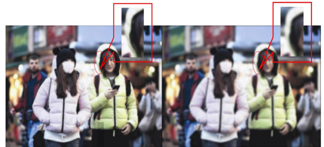
FIGURE 5. A sample image from prepared dataset, Left: main image - Right: after convolving with Gaussian filter of Eq. 8.
