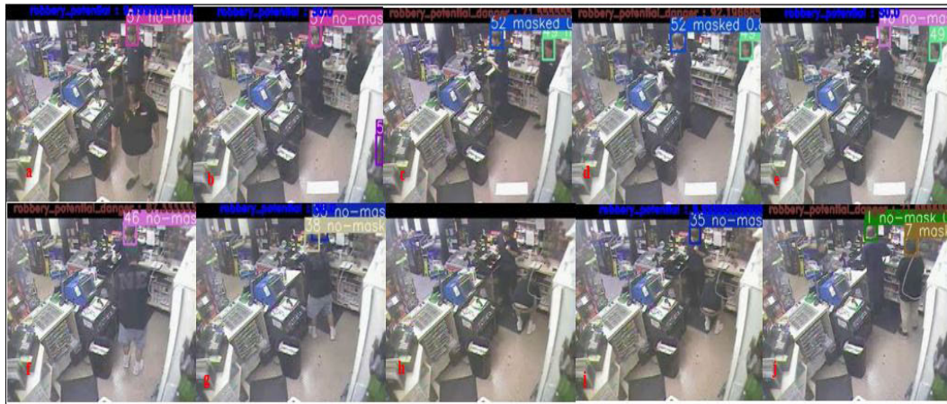
FIGURE 16. Sample of FN videos for robbery potential prediction. Calculated robbery potential of this sample is less than defined threshold but robbery happens at the end. Angle of camera can not cover the scene and human can not be detected.
