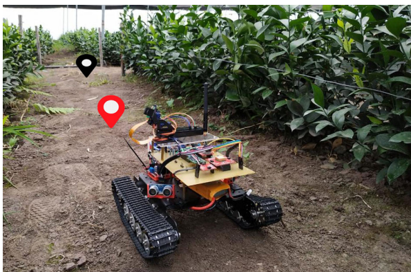
FIGURE 8. Prototype of the proposed-smart-farming robot while collecting data in a greenhouse.
