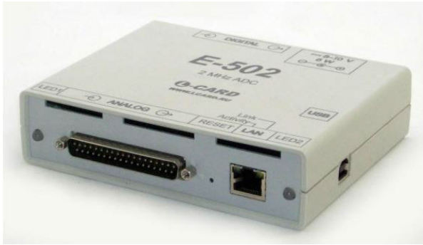
FIGURE 6. Appearance of the multifunctional ADC/DAC module E-502-P-EU-D.
