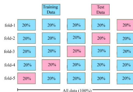
FIGURE 20. Illustration of the 5-fold method used to evaluate the effectiveness of the proposed method.
