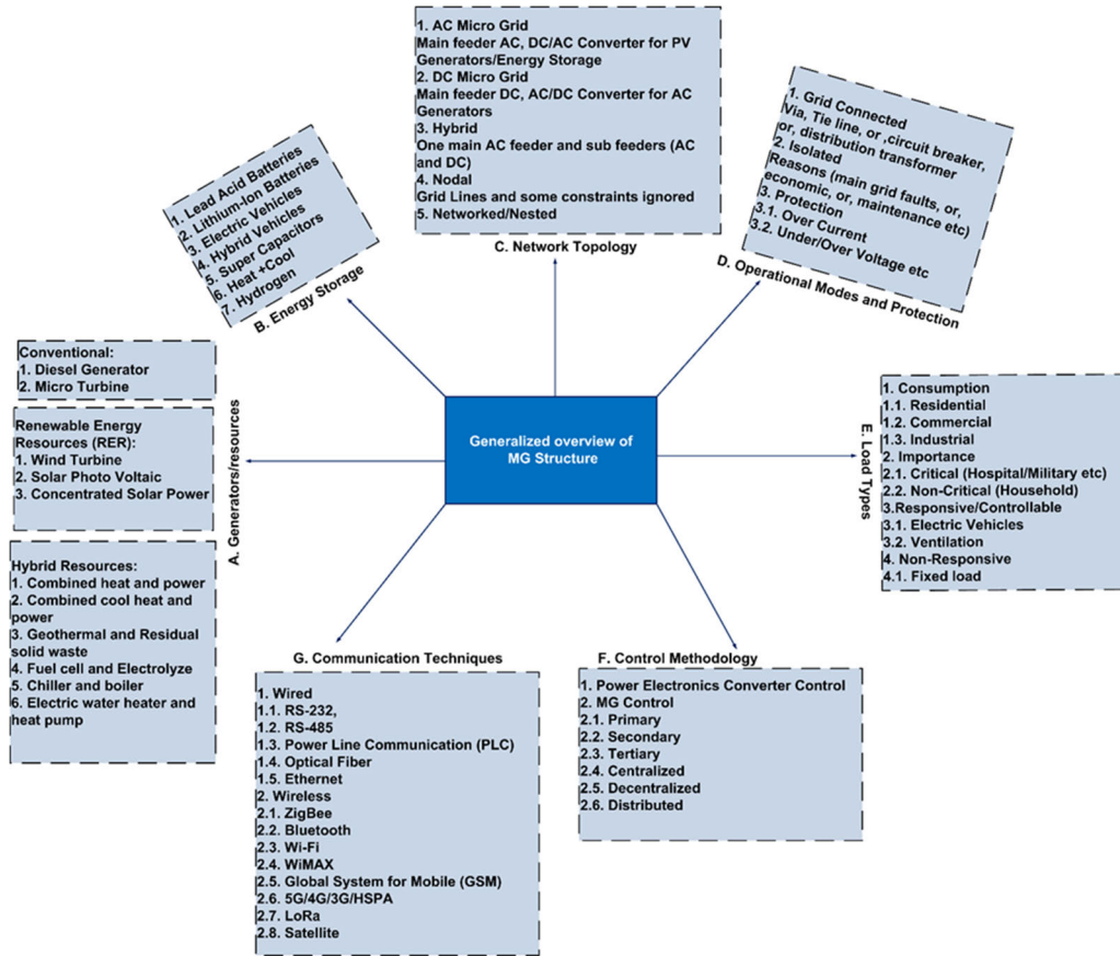
FIGURE 4. Generalized overview of micro grid structure.
