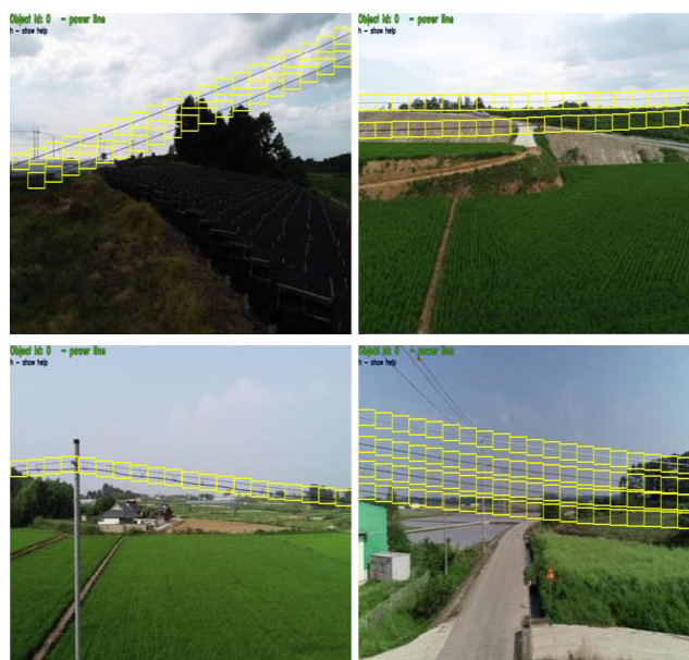
FIGURE 2. Labeling using a bounding box of size 0.05 times the size of the image.
