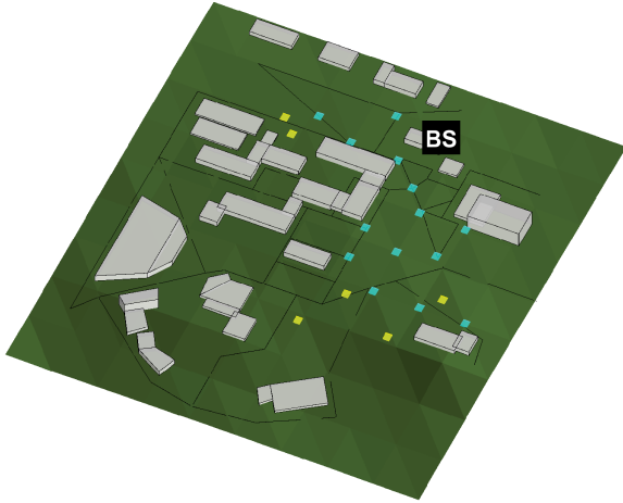
FIGURE 23. Six UEs are designated by yellow color for the first experiment. A total of 20 UEs, identified by both yellow and cyan colors, are employed for the second experiment.
