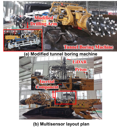
FIGURE 4. Hardware. The modified drilling arm was attached to the right side of the TBM. All sensors were mounted in the middle of the TBM. The LiDAR was located above the inertial component.
