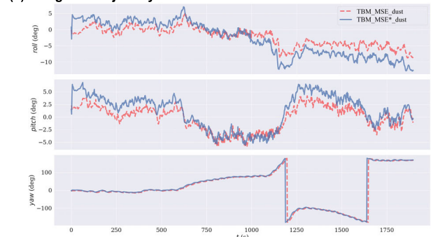
(b) Trajectory estimation of TBM-MSE and TBM-MSE* in three directions
