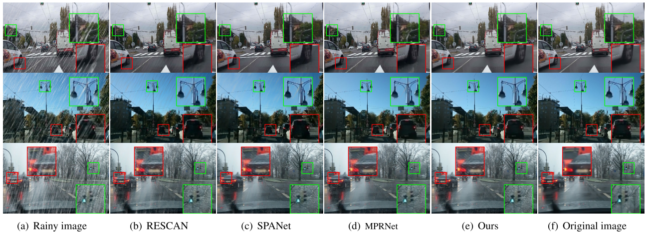
FIGURE 6. Comparison of rain removal results. The three rows from top to bottom represent light rain patterns, medium rain patterns, and heavy rain patterns. Each column from left to right represents the rain image, RESCAN deraining image, SPANet deraining image, MPRNet deraining image, our network deraining image, and the original image, respectively.
