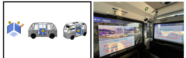
FIGURE 15. Installation of the screen inside the Navya shuttle. (Left) The blueprint of the screen installation. (Right) Actual installation of the two screens in perpendicular position.
