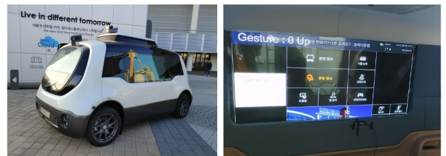
FIGURE 16. Installation of the screen inside the Robo shuttle. (Left) The outside view of the Robo. (Right) Actual installation of the screen inside the Robo shuttle.
