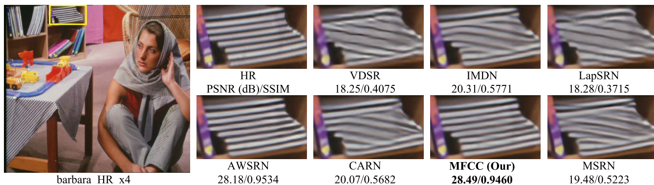
FIGURE 5. Qualitative comparison of barbara image belongs to Set14 dataset for scale \times 4 .
