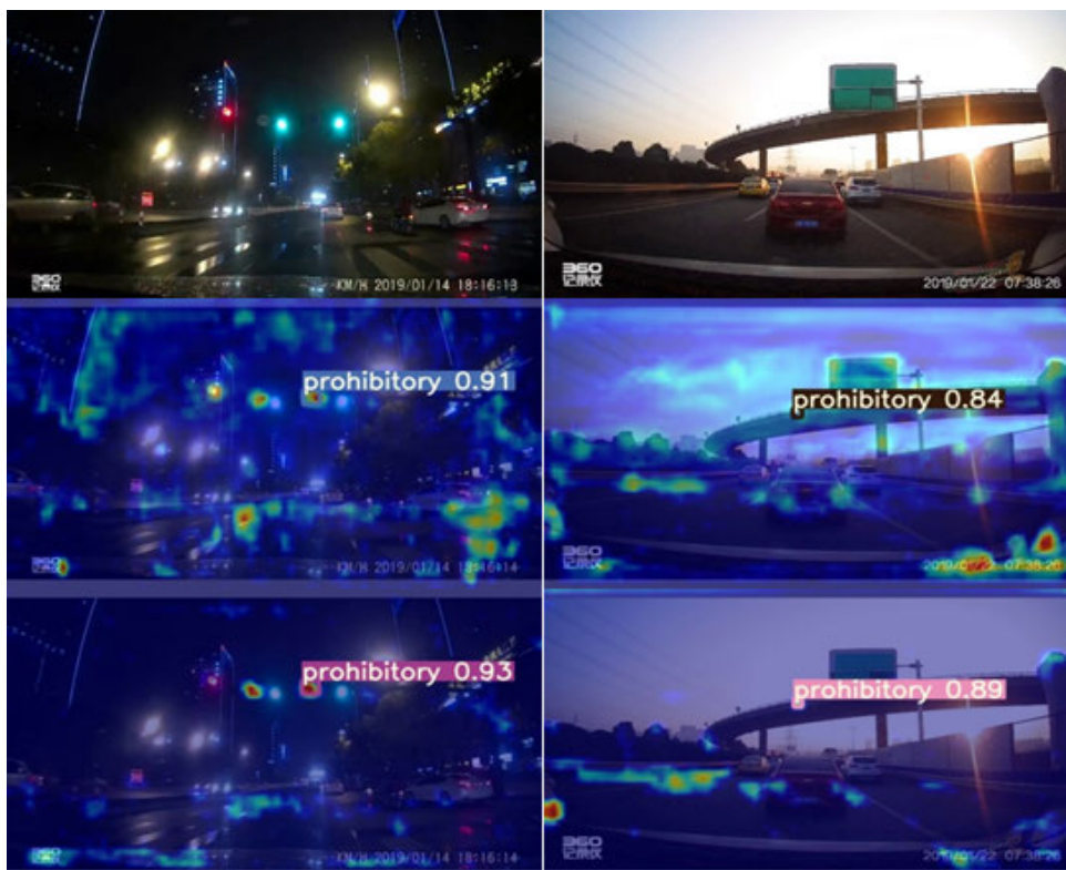
FIGURE 9. The first row are the original images, the second row are the thermodynamic diagram without CA model, and the last row are the results with CA model.
