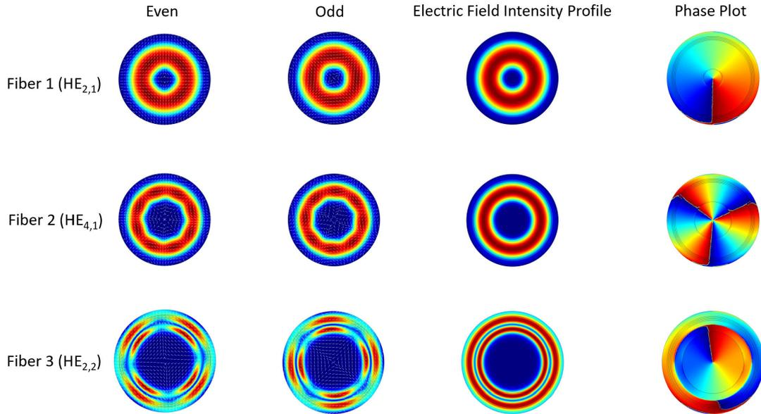
FIGURE 6. OAM mode generation and transmission for HE<sub>2,1</sub> in Fiber 1, HE<sub>4,1</sub> in Fiber 2 and HE<sub>2,2</sub> in Fiber 3.
