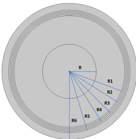
FIGURE 1. Schematic of proposed ring-core Bragg Fiber.
