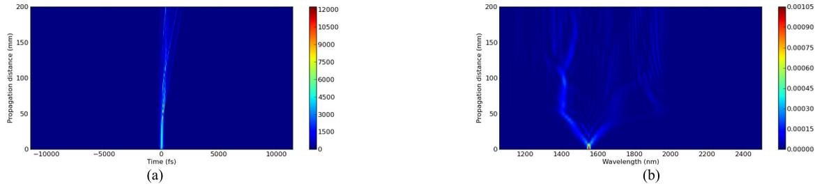
FIGURE 7. (a) Temporal and (b) Spatial domain evolution of 5 kW, 200 fs, 1.55 μm pulse in 20 cm RC-BF (Fiber 3).
