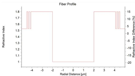
FIGURE 2. Index Profile of proposed ring-core Bragg Fiber.
