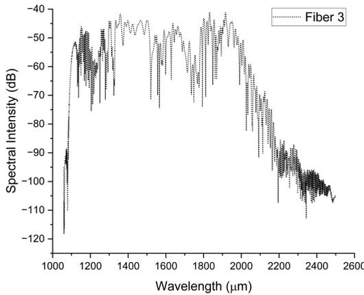
FIGURE 8. SC spectra at 20 cm fiber length.
