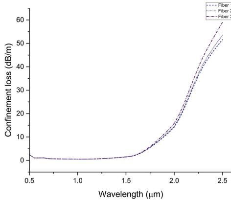
FIGURE 4. Confinement losses for Fibers 1, 2 and 3.
