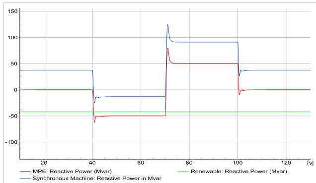
FIGURE 12. Reactive power control response profile with SC.
