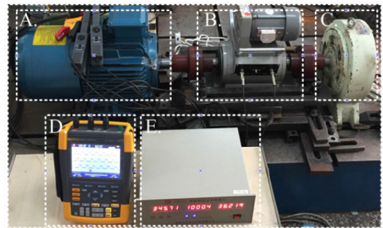
FIGURE 9. Prototype and experimental instruments. A. SRM prototype. B. Torque-speed measuring instrument. C. Magnetic powder brake. D. Wave recorder. E. Torque-speed indicator.
