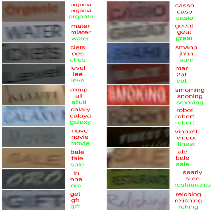
FIGURE 6. Comparison of outcomes on degraded images from the previous framework, such as 1) VisionLAN [31] and 2) ABINet [37] and the proposed framework. The recognition result strings of RMFPN are depicted beside each image. The first row and second row represent the output of ABINet and VisionLAN, respectively. Green characters are precisely predicted by our method.
