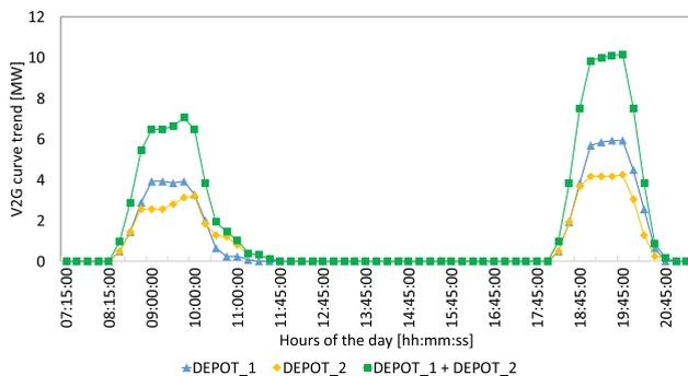
FIGURE 8. Electrical power provided to the grid using V2G service during weekdays.
