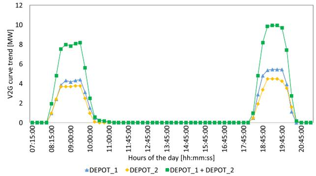
FIGURE 9. Electrical power provided to the grid using V2G service during Saturday.
