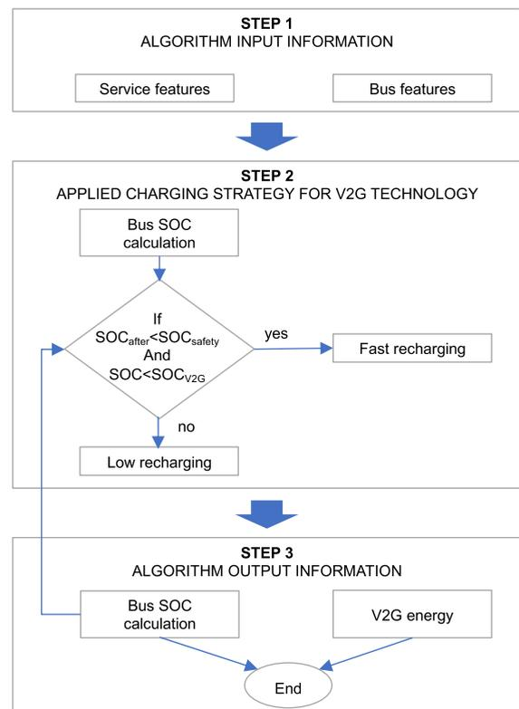
FIGURE 4. Flow-chart of the V2G proposed model.
