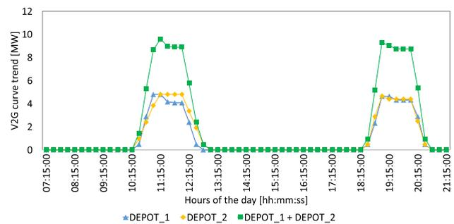
FIGURE 10. Electrical power provided to the grid using V2G service during holidays.
