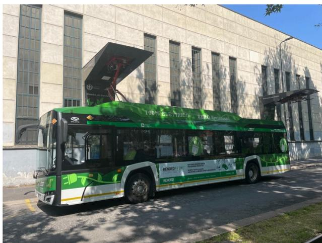
FIGURE 5. Electric bus model (12 meters long) and example of opportunity charger (pantograph) in the terminal used by LPT company.
