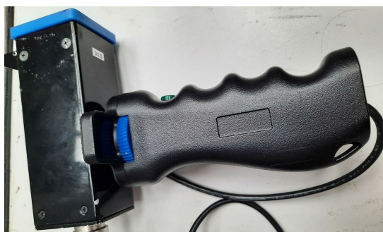
FIGURE 9. EVOTIS Instrumented Tap Testing device features a square faced contact aperture to ensure the strike is normal to the surface, consistent force application, and collects both force and sound time histories.
