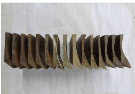
FIGURE 4. 15 test bulldozing plates.
