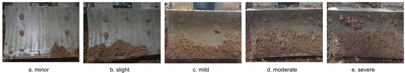
FIGURE 7. Soil adhesion evaluation criteria diagram.
