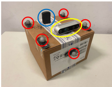
FIGURE 5. Positioning target in a real-world dataset. The yellow and blue circles mark the camera and UWB tag, respectively, and the five red circles indicate the Vicon ball for ground-truth estimation.
