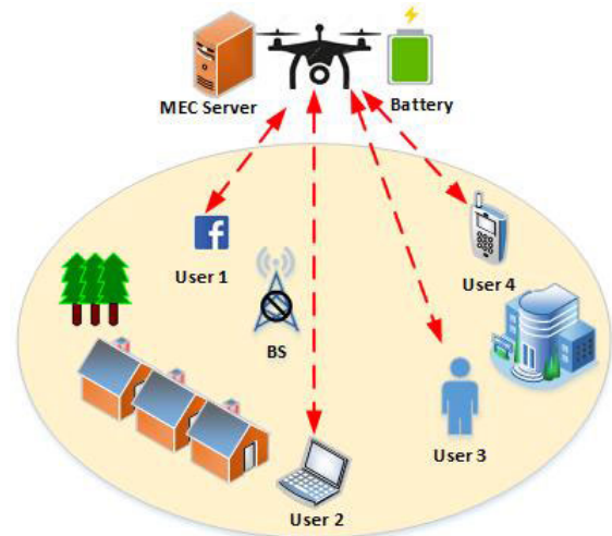
FIGURE 1. Interconnection of EuDs in UAV-MEC Network.
