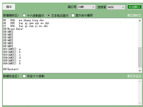
FIGURE 25. The voice command is written into the LD3320 in the form of Pinyin string through the upper computer.
