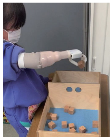
FIGURE 16. The child performing the box and blocks test using the developed prosthesis.
