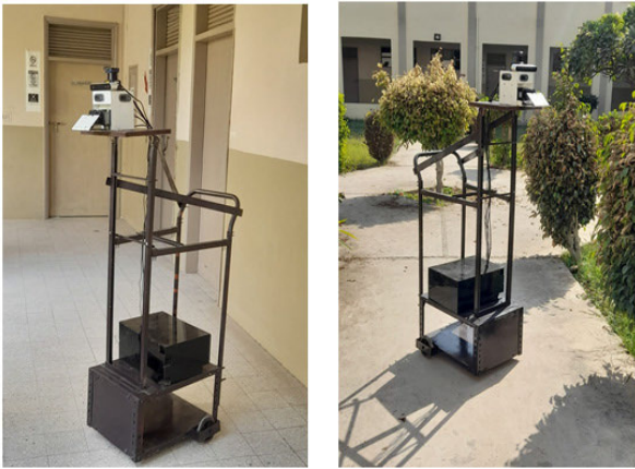
FIGURE 1. Custom made trolley based laser scanning system.
