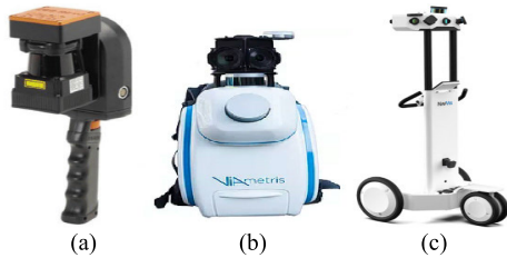
FIGURE 2. (a) ZEB REVO hand held (b) Viametris bMS3D LD5+ back pack (c) NavVis M6 mapping trolley systems.
