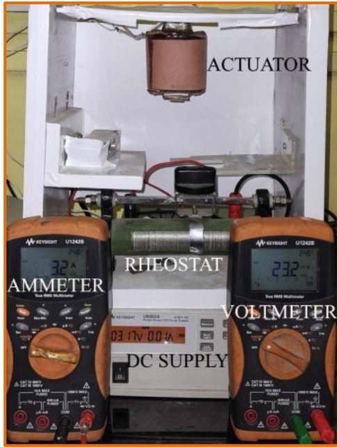
FIGURE 28. Hardware setup for resistance measurement for I-type actuator.
