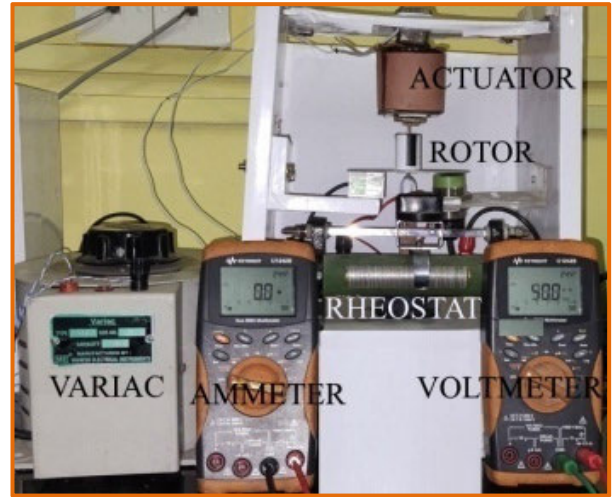
FIGURE 30. Experimental setup for inductance measurement for I-type actuator.
