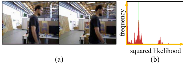
FIGURE 4. Histogram H in noisy scenes. (a) The sample of consecutive scenes. (b) Histogram of squared residual motion likelihood. The red lines are the frequency at each likelihood. The green line are the location of the median in the histogram.
