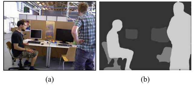
FIGURE 5. SSD probability. (a) RGB image. (b) Calculated SSD probability. Compared to the monitor, chairs and people appear brighter. This indicates that these objects are more dynamic than monitors.
