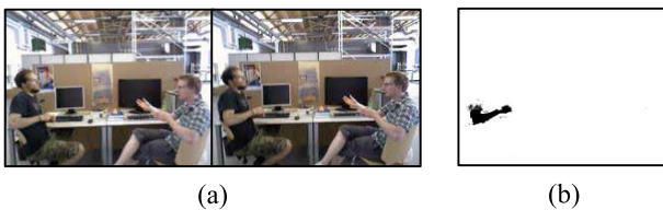
FIGURE 9. Example of good performance in sitting xyz sequence, (a) The sample consecutive scenes. (b) Post-processed GDM probability. Only the dynamic arms of the human body are expressed in black.
