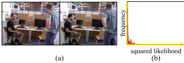
FIGURE 3. Histogram H in typical situations. (a) The sample of consecutive scenes. (b) Histogram of squared residual motion likelihood. The red lines are the frequency at each likelihood. The green lines are the location of the median in the histogram.
