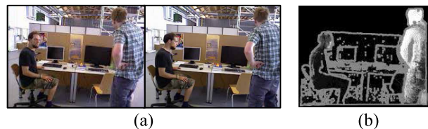
FIGURE 2. GDM probability. (a) The sample of consecutive scenes. (b) Calculated GDM probability: the brighter it is, the more dynamic it is.
