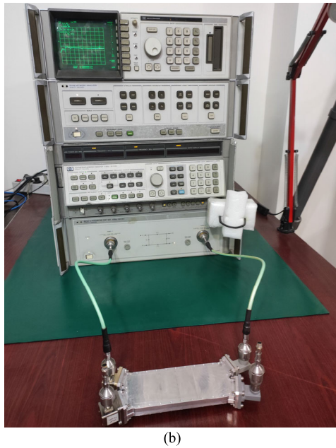
FIGURE 18. (a) Fabricated RGW-based three-section branch-line coupler, and (b) measurement setup.
