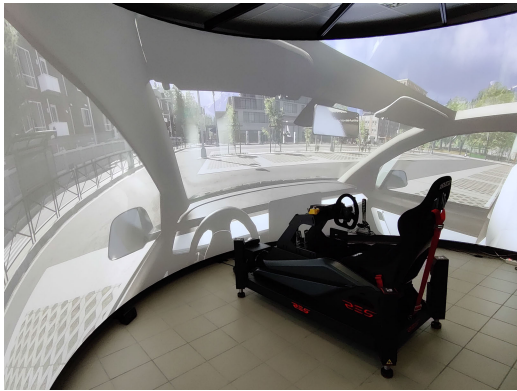
FIGURE 1. Vehicle driving simulator in the Autonomous Driving Laboratory of the University of Trento (Italy). The simulator implements the presented VS model in a real-time hardware.
