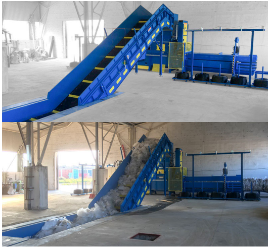
FIGURE 1. Belt conveyor for waste management [8].
