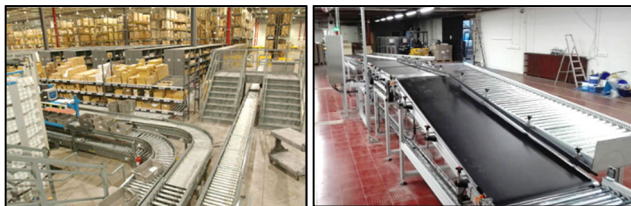
FIGURE 14. Examples of the areas for setting-up conveyor: multi-bended style (left), and straight pattern (right) [77], [78].
