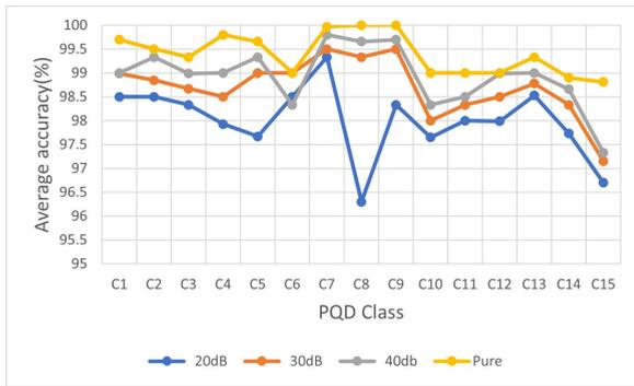
FIGURE 8. Classification accuracy of PQ events (%) with different values of SNR.
