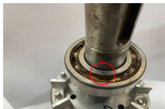
FIGURE 12. Bearing damage condition.
