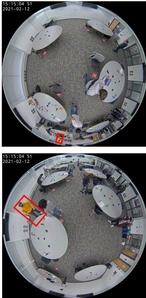
FIGURE 3. Illustration of the importance of color information in fisheye PRID. The person in the red bounding box in the top frame is severely shrunk, however the distinctive color of the sweatshirt still allows to distinguish this person from others.
