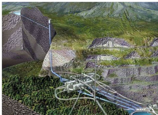
FIGURE 7. Side cut of Dinorwig PHS station [64].
