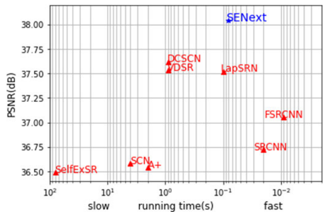
FIGURE 11. Quantitative evaluations of PSNR versus running time on Set5 with enlargement factor \times 2 .
