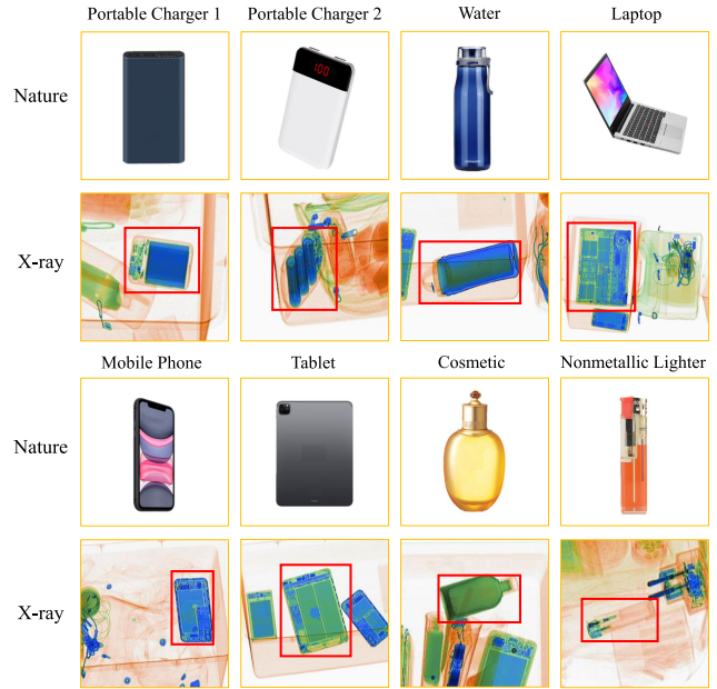
FIGURE 10. Different imaging demonstrations of the same objects under natural light and X-rays [92].
