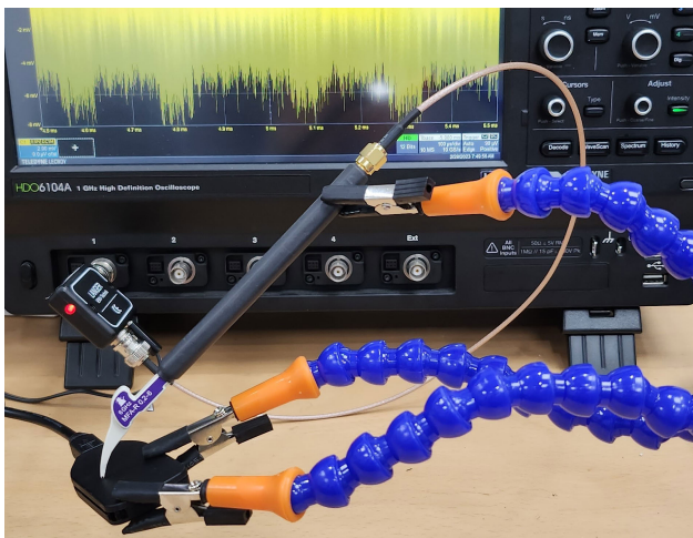
FIGURE 6. Power acquisition setup for the Real dataset.
