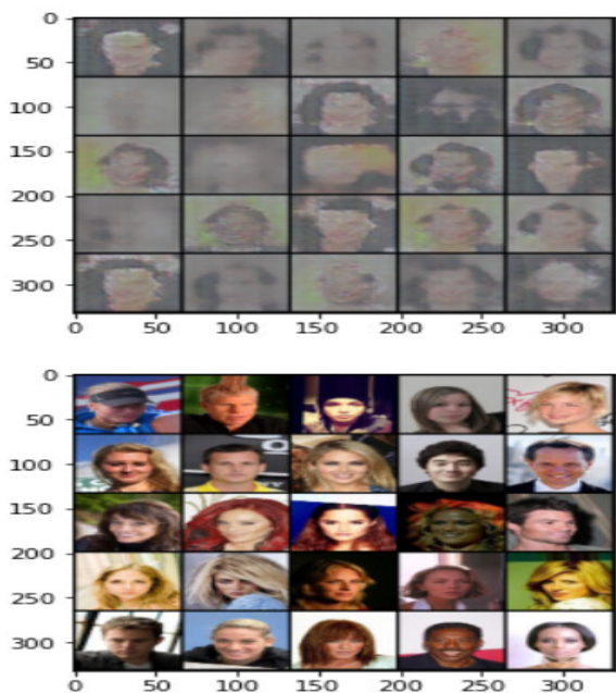
FIGURE 9. Visual output of the StyleGAN in the 10th epoch.
