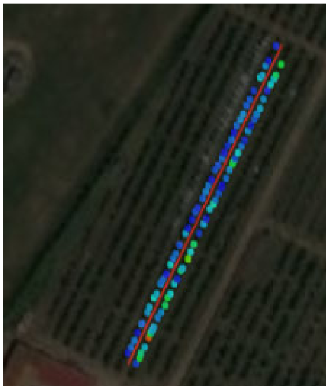
FIGURE 14. Representation of the trajectory and the canopy volume calculated for the upper section of trees.
