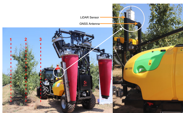
FIGURE 2. Tractor and sprayer used for data collection (left). Identify of the 2D LiDAR sensor and GNSS antenna (right). Line 3 in the left image represents the canopy area closest to the sensor. Line 2 marks the tree trunk, and line 1 represents the canopy area furthest from the sensor.
