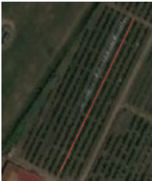
FIGURE 11. Representation of the trajectory performed by the sprayer.
