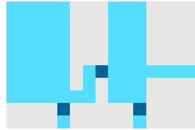
FIGURE 6. Circuit corresponding to bit string “1001011001000001000100”. The conductor paths between the input power port and capacitor 1 and those between the inductor and capacitor 2 are not selected. To avoid disconnection, conductors spread over the board are assigned.
