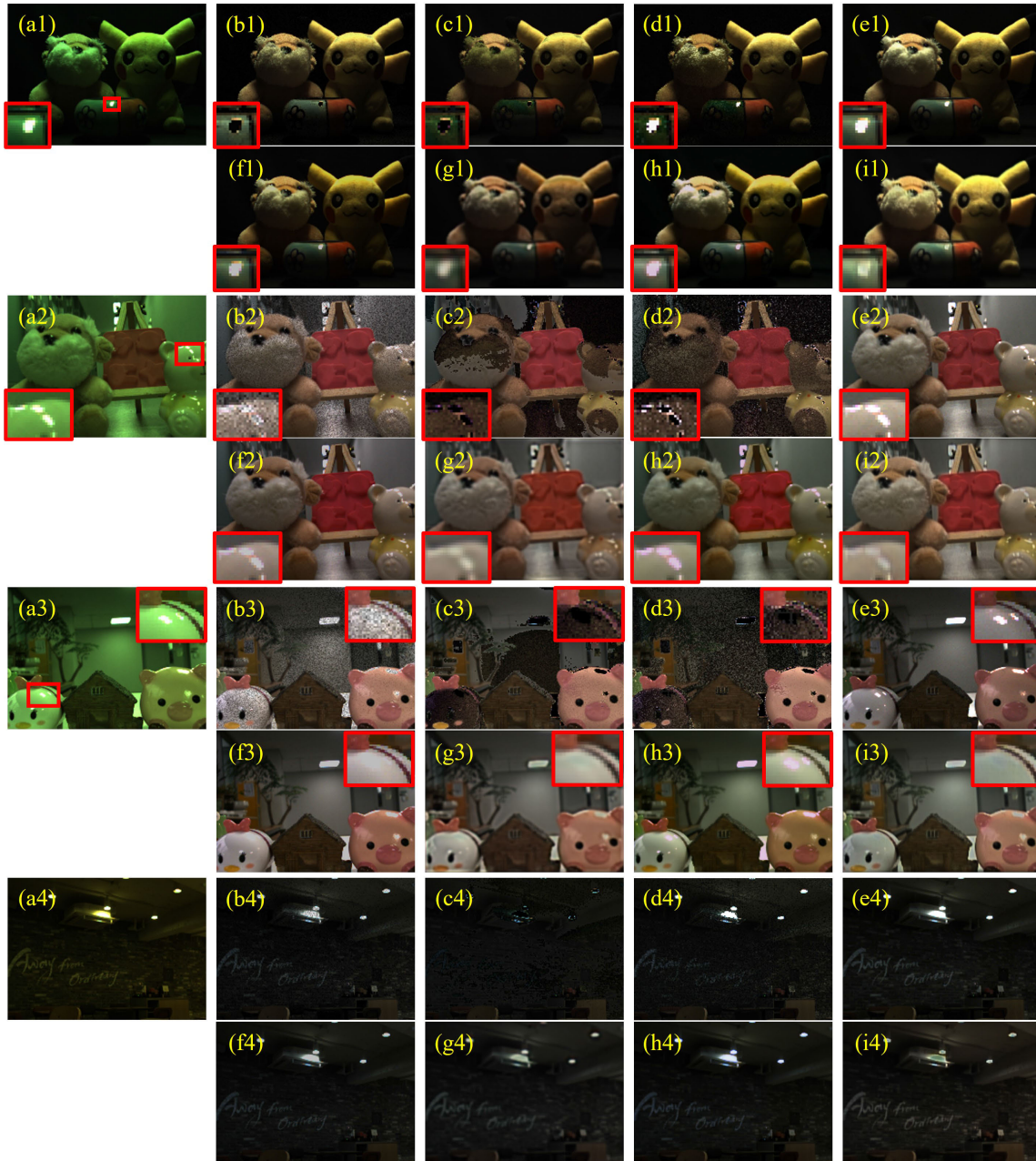
FIGURE 6. The dichromatic model results. (a) input image, the diffuse reflection of (b) Akashi et al. [13], (c) Yamamoto et al. [14], (d) Yang et al. [58] (e) Tsuji [20], (f) Fu et al. [16], (g) JSHDR [57], (h) DDME [6] and (i) the proposed method.
